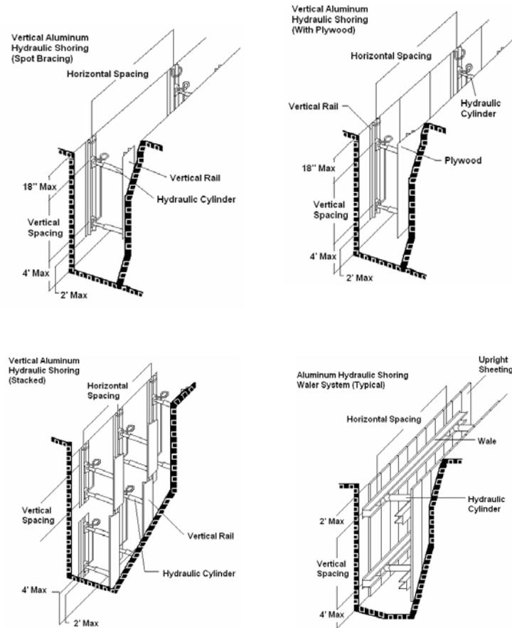
**ALWAYS INSTALL SHORING FROM THE TOP DOWN AND REMOVE FROM BOTTOM UP**
