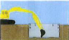
EXCAVATE UNTIL SOIL BEGINS TO CRUMBLE BEYOND DESIRED TRENCH WIDTH. PLACE SHIELD IN LINE OF EXCAVATION
