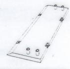
Place one sidewall flat on the ground with collars pointing up.
