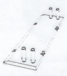
Set the spreader pipes over the collars and insert pins and keepers.
