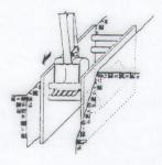
Pull shield forward by front spreaders or pulling eyes. Continue excavating and pulling shield forward as work progresses. Backfill as work proceeds.
