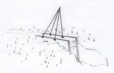
WARNING: Lift eyes are designed and intended for assembly and lifting only. Do not pull or lift by eyes when shied is stuck or has pressure against it. Loosen shield by pulling on spreader bars or digging along sides before using lift eyes.
