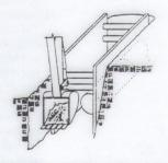
Perform desired work, then excavate in front of shield.
