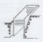
Excavate trench to grade, slightly wider than shield. Lift and lower shield into trench.
