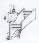
Continue excavating within shield while alternately pushing down on corners, until proper grade is reached.
