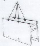
Place sling in top 4 lift lugs. Stand shield and install into trench.
