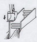
Continue excavating within shield while alternately pushing down on corners, until proper grade is reached.
