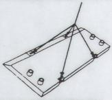
Remove from truck by lifting panels with 4 point lift lugs. Always use OSHA approved slings.
