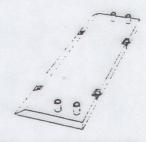
Place one sidewall flat on the ground with collars pointing up.
