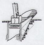
Perform desired work, then pull shield forward and up at appropriate angle and repeat steps (2) and (3) as necessary. Backfill as work progresses.
