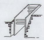
Excavate trench to grade, slightly wider than shield. Lift and lower shield into trench.
