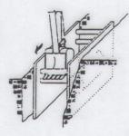
Pull shield forward by front spreaders or pulling eyes. Continue excavating and pulling shield forward as work progresses. Backfill as work proceeds.
