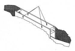
WARNING: Lift eyes are designed and intended for assembly and lifting only. Do not pull or lift by eyes when shield is stuck or has pressure against it. Loosen shield by pulling on spreader or digging along sides before using lift eyes.
