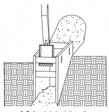
Perform desired work, then pull shield forward and up at appropriate angle and repeat steps (2) and (3) as necessary.
