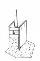
Excavate until soil begins to crumble beyond desired trench width.
