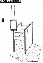
Continue excavating with in shield while alternately pushing down on shield corners, until proper grade is reached.
