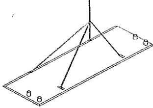
1. Remove from truck by lifting panels with 4 point lift lugs. Always use OSHA approved slings.
