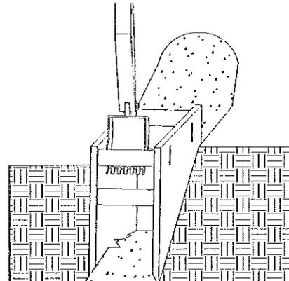
3. Perform desired work, then pull shield forward and up at appropriate angle and repeat steps (2) and (3) as necessary.
