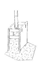
Excavate until soil begins to crumble beyond desired trench width, Place shield on line of excavation and excavate from within,
