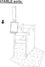
Continue excavating with in shield while alternately pushing down on shield corners, until proper grade is reached.
