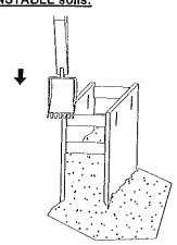
Continue excavating with in shield while alternately pushing down on shield corners, until proper grade is reached.
