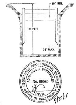
2" DIAM. PINS SHALL HAVE MIN Fu = 92 KSI. CONTRACTOR RESPONSIBLE FOR ENSURING PROPER GRADE PINS ARE IN PLACE PRIOR TO SHIELD USE.
