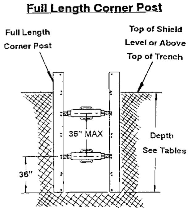
NOTE: Alternate installation and trenching methods shown on sectional corner posts also apply
