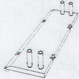
3. Set the spreader pipes over the collars and insert pins and keepers.
