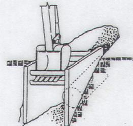
3. Perform desired work, then pull shield forward and up at appropriate angle and repeat steps (2) and (3) as necessary. Backfill as work progresses.
