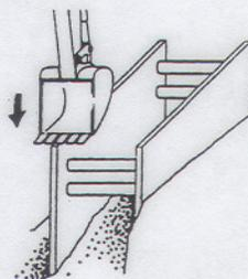
2. Continue excavating within shield while alternately pushing down on corners, until proper grade is reached.
