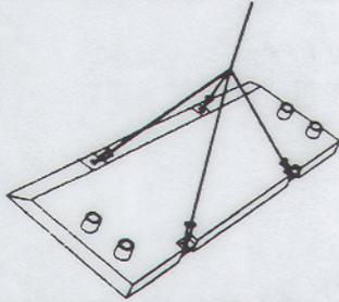
1. Remove from truck by lifting panels with 4 point lift lugs. Always use OSHA approved slings.
