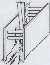
1. Excavate until soil begins to crumble beyond desired trench width. Place shield on line of excavation and excavate from within.
