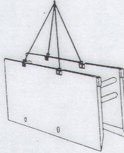
5. Place sling in top 4 lift lugs. Stand shield and install into trench.
