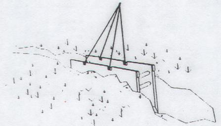
6. **WARNING:** Lift eyes are designed and intended for assembly and lifting only. Do not pull or lift by eyes when shield is stuck or has pressure against it. Loosen shield by pulling on spreader bars or digging along sides before using lift eyes.
