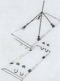
4. Set matching panel over bottom panel. Install spreader pipes in collars and insert pins and keepers.
