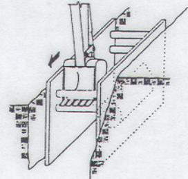
3. Pull shield forward by front spreaders or pulling eyes. Continue excavating and pulling shield forward as work progresses. Backfill as work proceeds.
