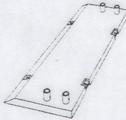
2. Place one sidewall flat on the ground with collars pointing up.
