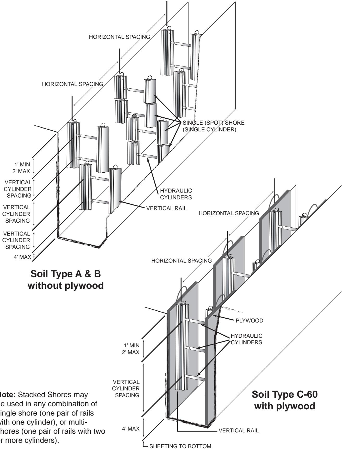
**Note:** Stacked Shores may be used in any combination of single shore (one pair of rails with one cylinder), or multi-shores (one pair of rails with two or more cylinders).
