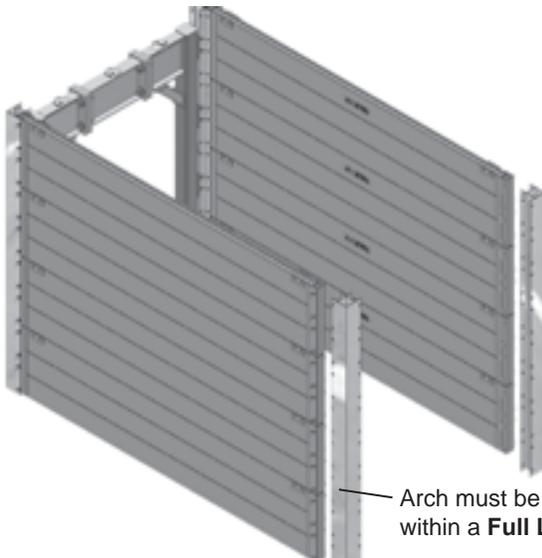
Arch must be pinned completely within a **Full Length** corner post.
