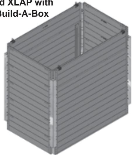
1. Corner Posts must extend a minimum of 1 ft. both below and above the intersection of the Build-A-Box panel on the XLAP Aluminum Trench Shield
