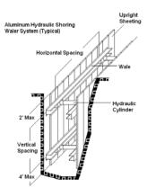
ALWAYS INSTALL SHORING FROM THE TOP DOWN AND REMOVE FROM BOTTOM UP
